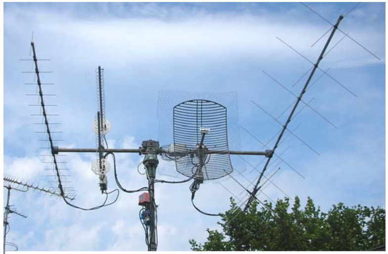
Figure 1. OZ1MY antennas. From left to right, 70 cm 2x19 element Tonna, 2 19 turn helixes for 23 cm, BBQ dish for 13 cm and 2x9 element 2 meter antenna, Tonna.
