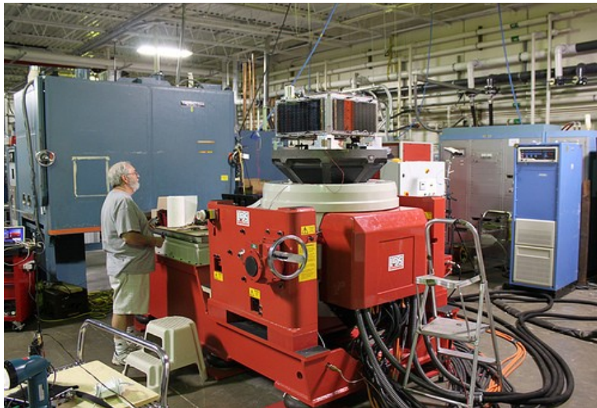
ARISSat-a under vibrationstests.
